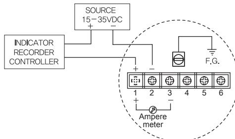
※ You can check 4-20mA output by connecting an ampere meter. (impedance: max. 30Ω)
