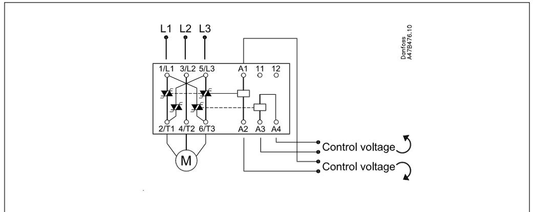
**Motor overload and short circuit protection**
